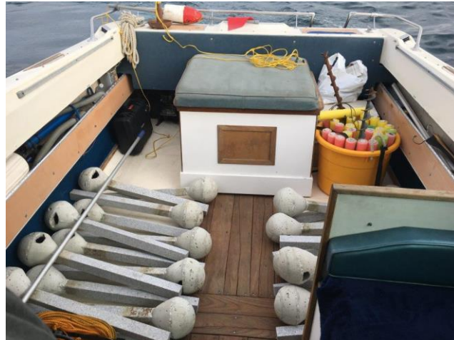
The Amanda II loaded with octo columns, descenders, augers, mushroom anchors and buoys.
