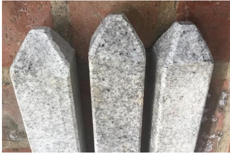
Columns with tapers cut on top to reduce tendency of sediment to settle on top.
