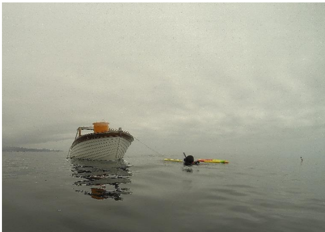
Multiple descenders on surface. Each descender prussic loop was threaded onto the water jet hose and they eventually worked their way to the surface. Note marker buoy in right of photo.
