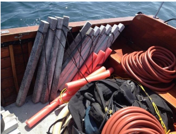
Granite columns ready to deploy with descenders attached using prussic loops.
